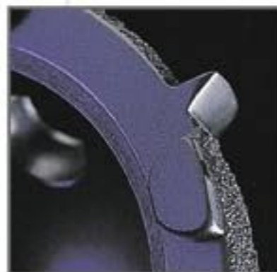
The RingLoc acetabular shell is designed with four anti-rotational fins that engage the superior rim, the pubis and the ischium for initial stability. A metal ring washer securely locks the liner into the shell and peripheral tabs keep the liner rotationally stable.
