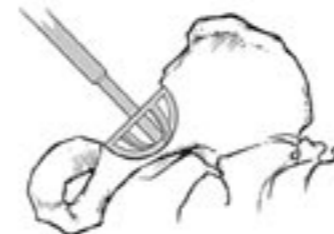
A trial metal frame shell gauge is used to determine the final shell diameter.
