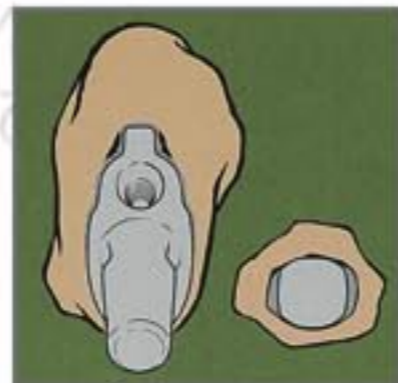
Quadrilateral fixation is illustrated showing maximum canal filling in the proximal region. The distal cross-section shows how the Mallory-Head porous stem fills the canal and allows for close contact of the stem to bone.
