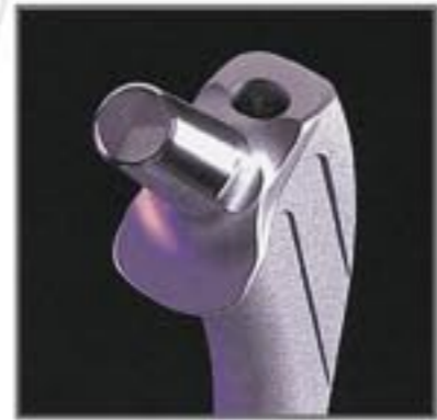
The Mallory-Head Intelok prosthesis offers an enhanced proximal design to promote increased proximal loading. This is achieved through a latera-to-medial taper augmented with anterior and posterior "ribs" angled at 20 degrees to help force cement into compression medially. The entire proximal geometry features an Intelok roughened surface for increased cement/stem fixation.
