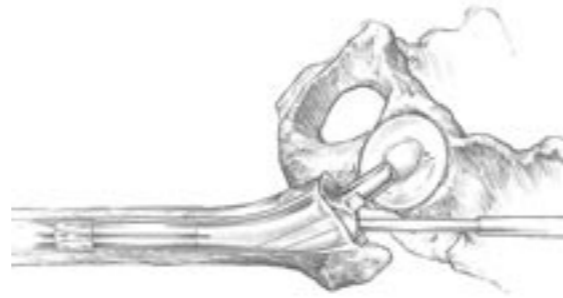
The centering sleeve provides for an even cement mantle distally. Parallel ribs enhance proximal fixation.
